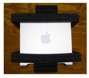
**Step 3a:** Take the cardboard corner shims and slide them between each corner of the foam protectors and the edge of the Mac Pro. This prevents foam tearing.
