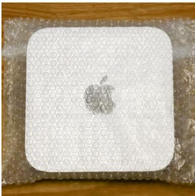
3. Tuck the excess bubble wrap under the Mac mini, then set it inside the cut-out so it sits flush with the top of the foam.
